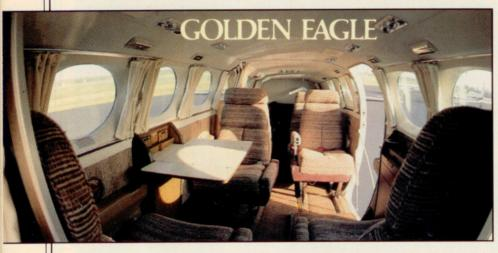
be accomplished before each flight. A well-equipped Golden Eagle can carry more than 2,000 pounds of fuel, people and baggage; and the pilot must ensure that the airplane does not exceed the maximum certificated zero-fuel weight (6,733 pounds), maximum ramp weight (7,500), takeoff weight (7,450) or landing weight (7,200 pounds).
